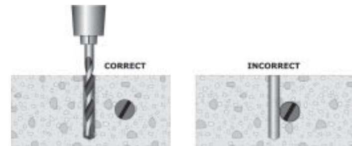
Figure 130: Drilling into concrete with rebar.
