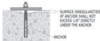
Figure 134: Acceptable gap for grouted plate.
