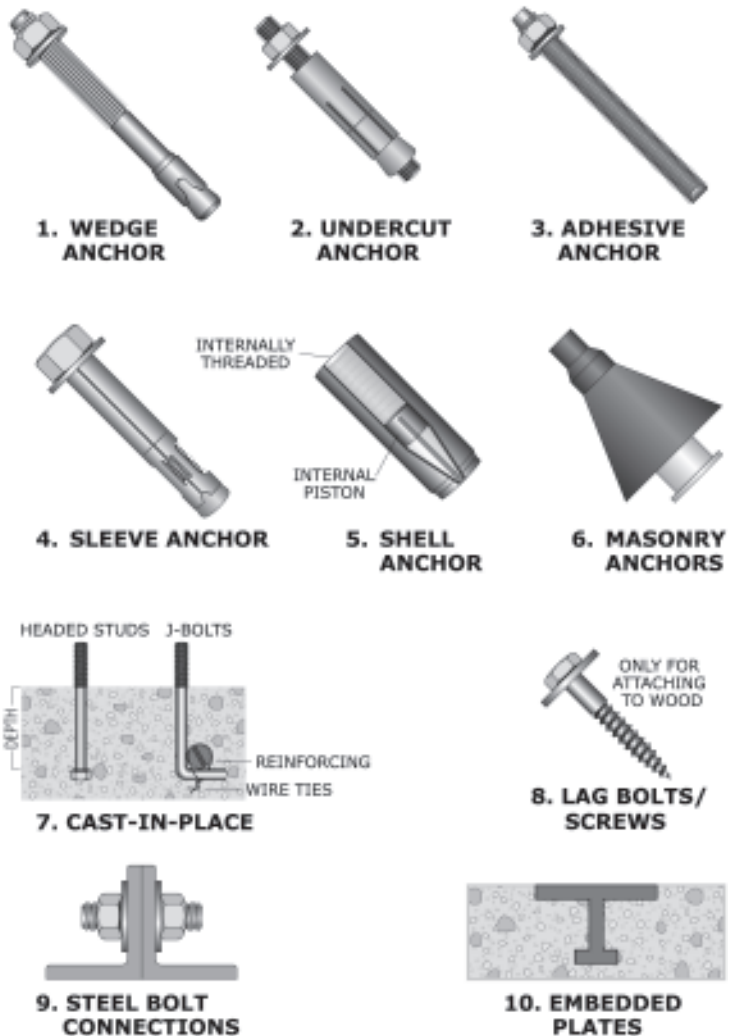
Figure 130: Types of anchors.
