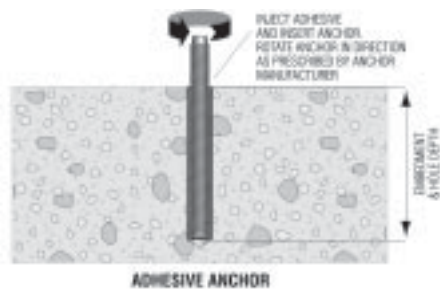
Figure 131: Adhesive anchor installation.
