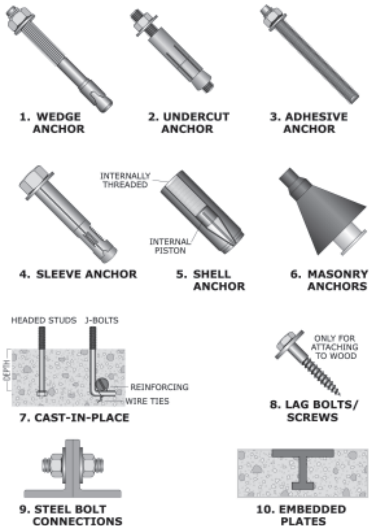
Figure 130: Types of anchors.
