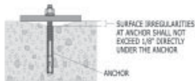
Figure 134: Acceptable gap for grouted plate.
