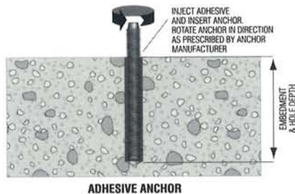
Figure 110: Adhesive anchor installation.
