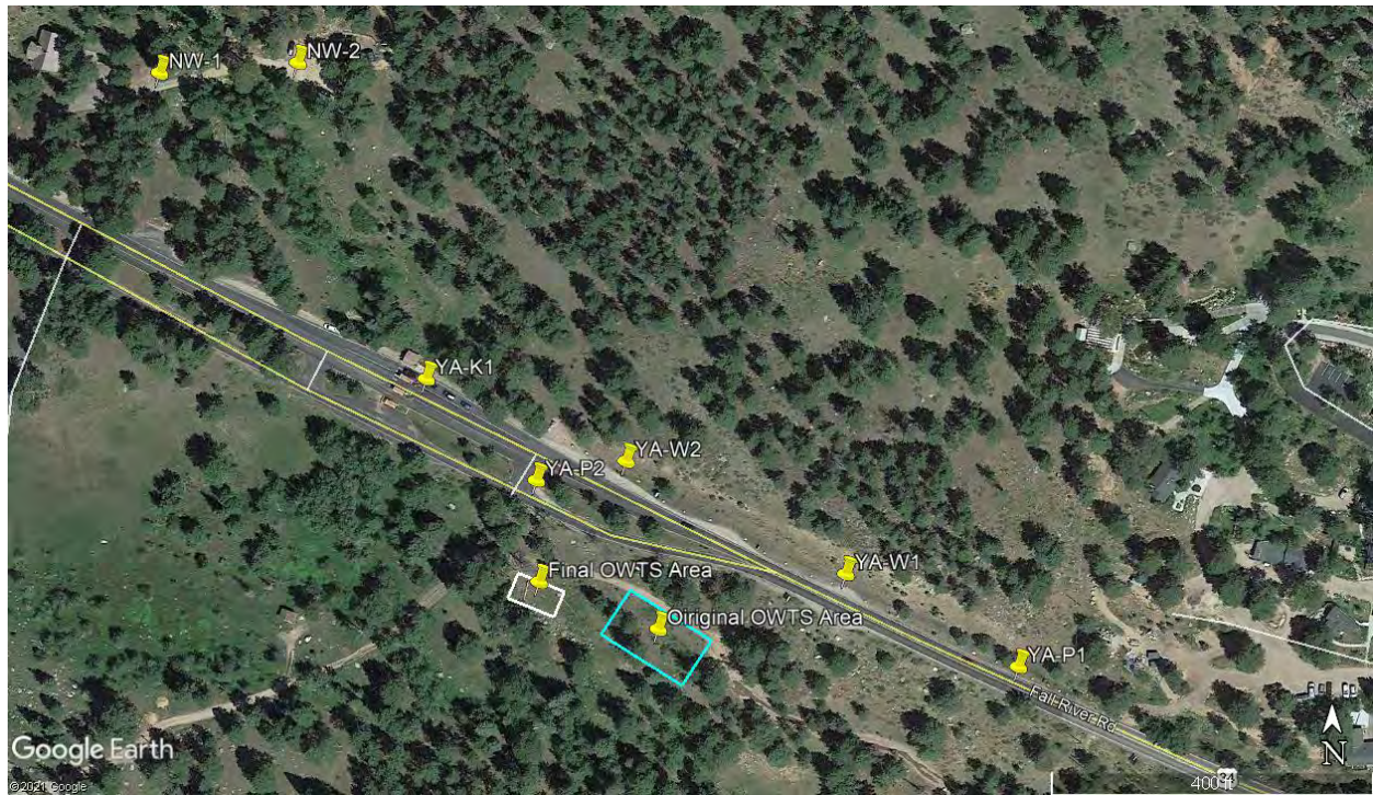
Figure 2. Approximate boring locations
