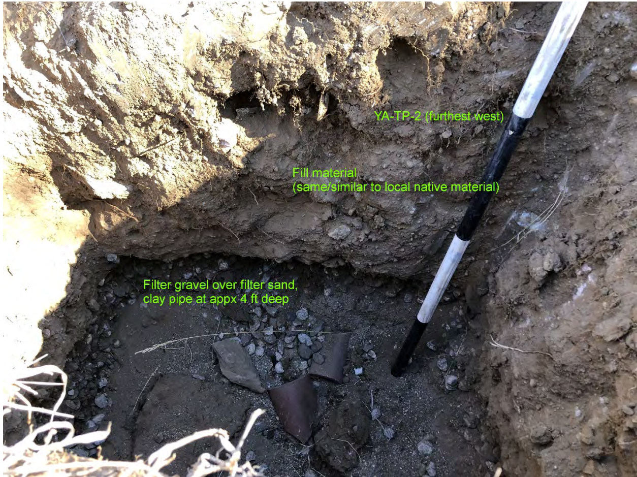
Figure A 2. Annotated image of test pit YA-TP-2 at original OWTS location.
