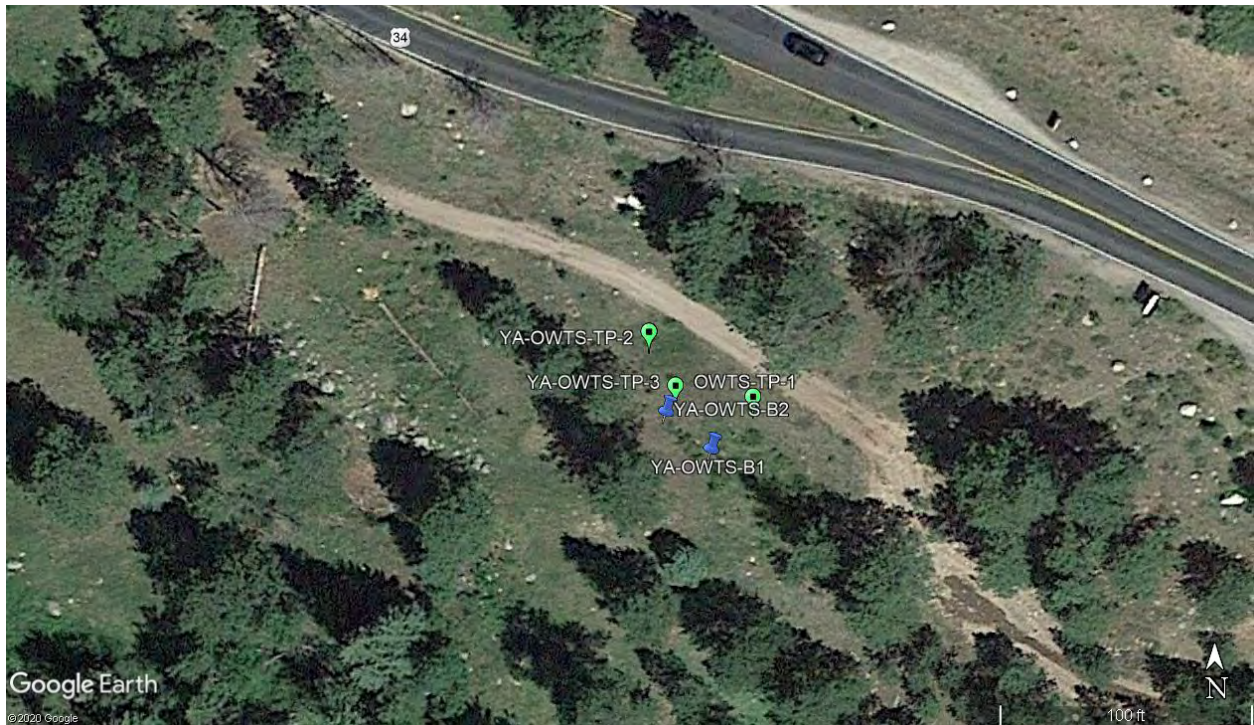
Figure 3. Approximate boring and test pit locations from the original OWTS investigation.
