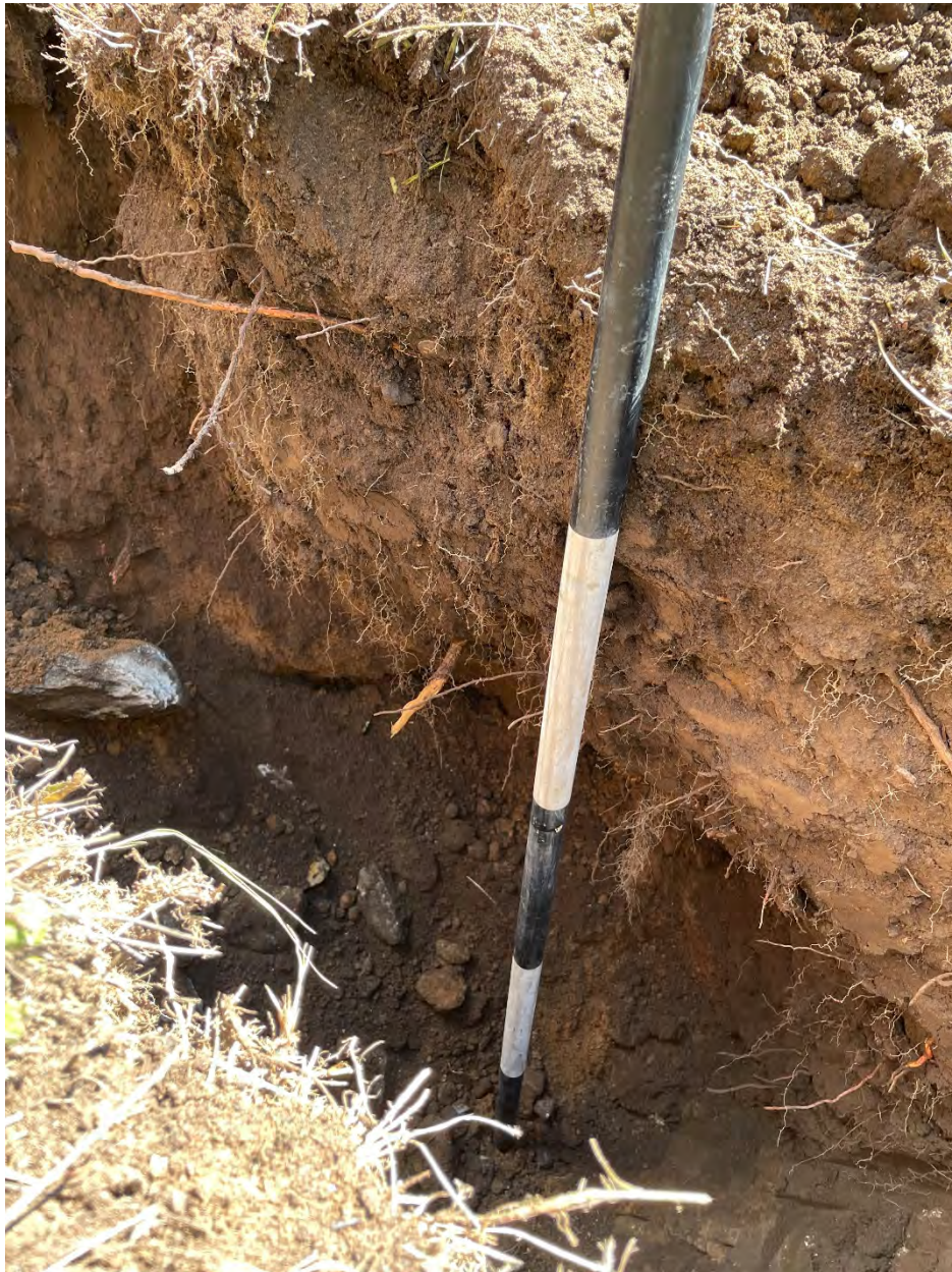
Figure A 4. Test pit YA-TP-1 at final OWTS location.
